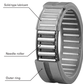
Structure of Capilube Bearing
